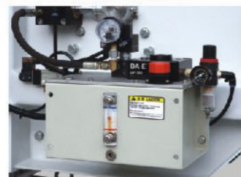
锯片的松紧度由气动/液压装置控制,在工作过程中,一旦出现压力下降的情况,气动部分可自动提供压力补偿,保证锯片的松紧度在任何时候都处于恒定状态。 Blade tightness controlled by pneumatic / Hydraulic device The blade tightness is controlled by pneumatic / Hydraulic device. In case hydraulic pressure drops, the air system provides a pressure compensation to ensure a constant blade tension at all time.
