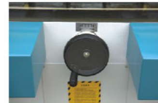
后台靠尺微调手轮及数字显示器，可精确显示剪切宽度。 Fine tuning ruler with indicator show exact cutting width.
